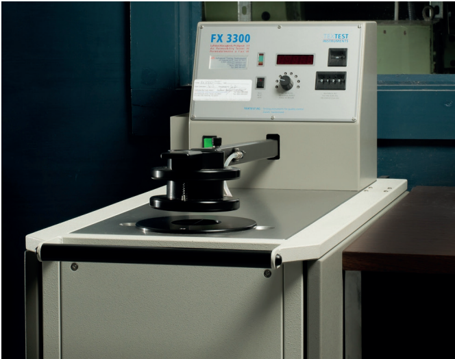
FIGURE 1. Traditional Permeability Tester uses a goose neck to reach inside the edges of a fabric.
