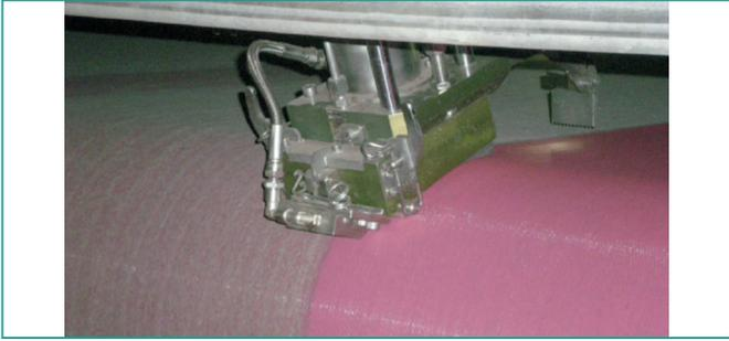
**MECHANICAL CLEANING.** Mechanical cleaning is the lowest cost method for cleaning dryer fabrics. The two most common mechanical cleaning methods include the use of rotating brushes and chain mesh to scrape heavy contaminants from the surface of the fabric (Figure 5). You should closely monitor these mechanical systems to prevent excessive abrasion to the dryer fabric's surface, which could lead to premature failure.
