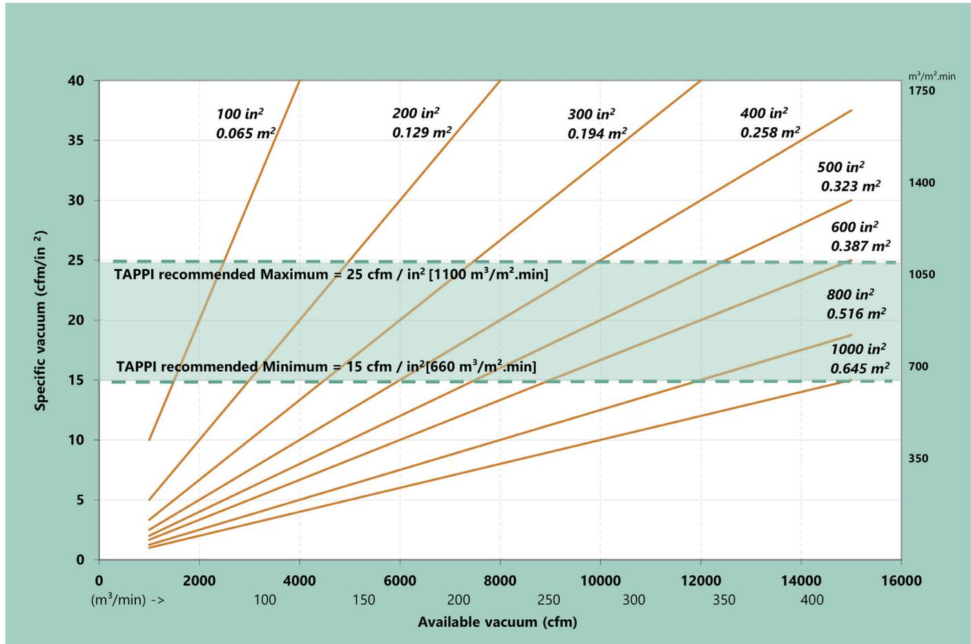
FIGURE 5. TAPPI guidelines for Uhle box vacuum density [modified after 1].
