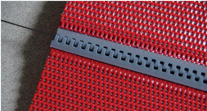
QuickLink replaces traditional weave-back loops in a dryer fabric seam with an innovative polymer-bonded seam. QuickLink loops line up easily, almost like a zipper. The seam is below the plane of the fabric, which eliminates a potential wear point and virtually ensures that the fabric will be non-marking on the sheet.
