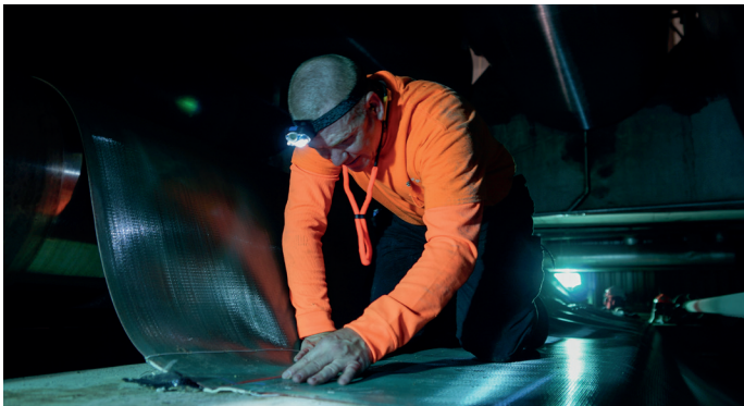
QuickLink enables machine crews to get in and out of the dryer section during a fabric change as quickly and safely as possible. IEP's first QuickLink fabric was installed on the 5th bottom position of No. 5 machine. The seaming was accomplished in a little over three minutes – compared to 10-12 minutes with traditional fabrics.
