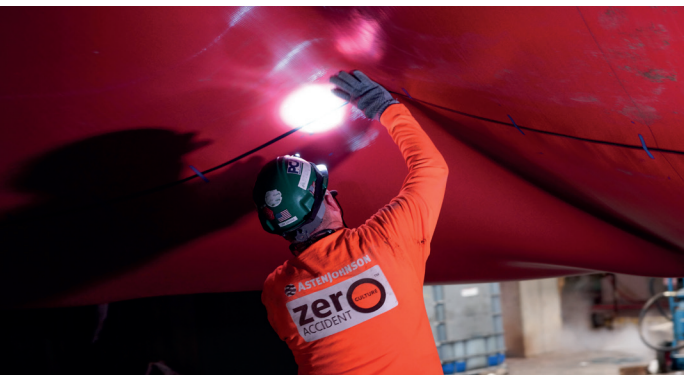
Jim Brink of AstenJohnson makes a final quick inspection of the QuickLink seam before the fabric is tensioned.
