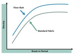
Finer batt closes the permeability and reaches optimal pressing moisture sooner but increases overall operating density.
