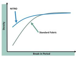
NITRO combines the effects of pre-compaction and using finer batt, without affecting late life density.
